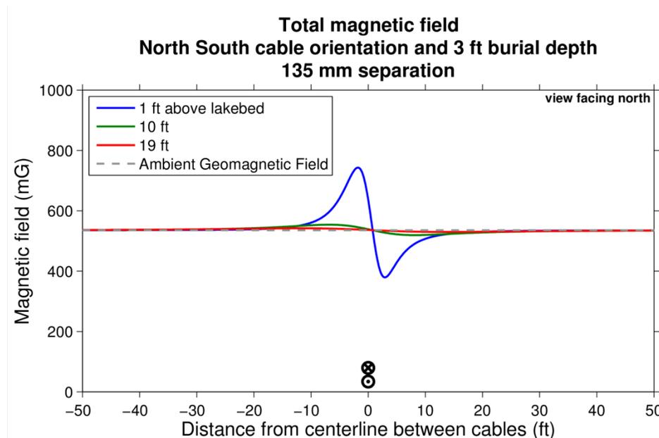
Figure 1. Case T. Magnetic field profiles (mG) above north-south oriented cables buried 3 feet, cables separated by 135 mm, and northward current in the top cable.
