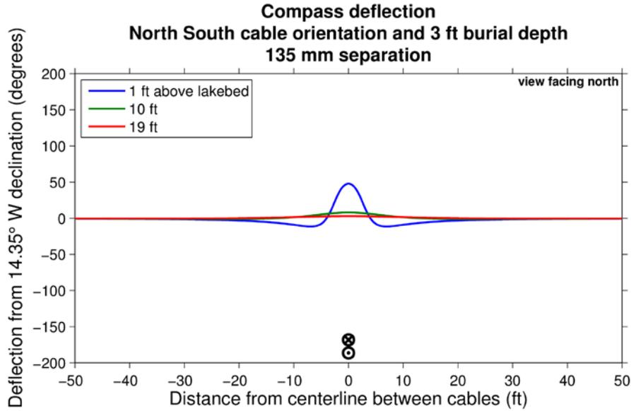
Figure 3. Compass deflection (degrees) from 14.35 degree W declination above north-south-oriented cables buried 3 feet, cables separated by 135 mm, and northward current in the top cable.
