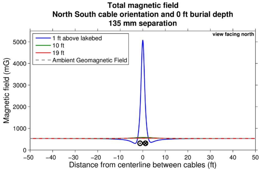
Figure 2. Case B. Magnetic field profiles (mG) above north-south oriented cables on the lakebed, cables separated by 135 mm, and northward current in the eastern cable.
